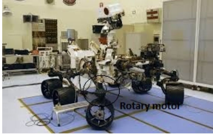
Figure 3.6: Independent Steering Using Rotary Motors [Courtesy: NASA/JPL]
