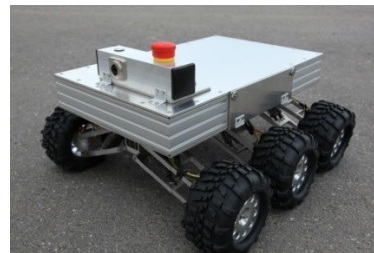
Figure 2.4: Six wheel independent spring suspension in All Terrain Vehicles and Robots
