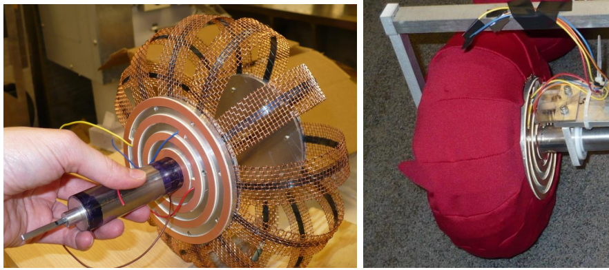
Figure 4.16: Reconfigurable wheel prototype developed at MIT [8]
