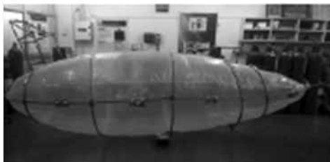
Figure 14 : Assembly of semi-rigid airship
