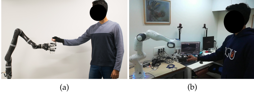
Figure 4.6: Setup for testing STL controllers for human-robot handovers with (a) Kinova Jaco-2 collaborative robot, (b) Franka-Emika Panda collaborative robot
