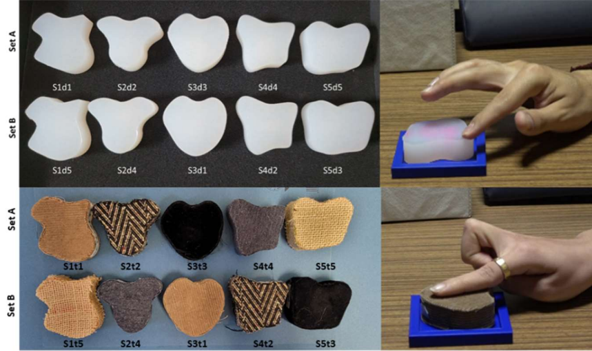
Fig. 1. Depiction of the experimental set-up, as well as the smooth-deformable shapes (top left panel) and textured-rigid shapes (bottom left panel) used in the experiment.
